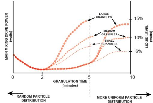
In Processall’s Mixmill® line of mixing granulators, medium density blending elements lift and disperse the product to produce a mechanically fluidized bed, which rapidly and efficiently blends materials of widely different density and particle size, while an integral high-intensity chopping mill system distributes the agglomerating solutions while binding and controlling particle size. Post milling is usually unnecessary.
